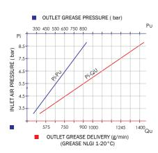
Those are suitable for central supply of plants where a major pressure at long and short distance is required. The operating pressure of the grease pumps hereby may vary between a minimum of 2.5 bar and a maximum of 8 bar. In order to optimize the efficiency and the life of our pneumatic pumps we recommend to use filtered and lubricated air.
